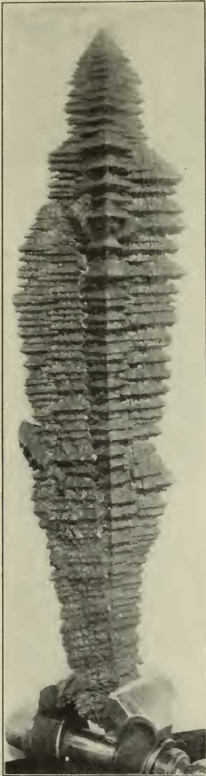
STEEL CRYSTAL, A LITTLE LESS THAN ONE-HALF NATURAL SIZE. COLLECTION OF PROF. TSCHERNOFF.
